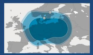
ASTRA 3B - Key Data Orbital location: 23.5°E Total transponders: Ka-band: 4 (250 MHz) Ku-band: up to 56 out of 40 BSS (33 MHz), 24 FSS (36 MHz)
